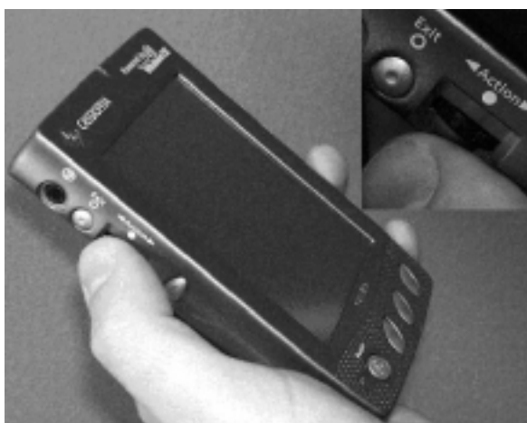
Figure 2. The Casio Cassiopeia E-11 with a close-up on the Action Control. The left-hand thumb of a right-handed user is positioned on the Action Control.
