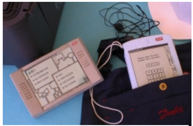
Second design iteration cycle: Two concepts left. System Style fits in toolbox, Tool Style in pocket
